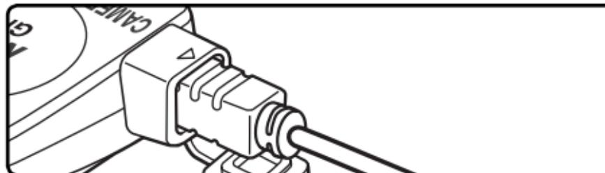
**3** Open the camera accessory terminal cover and insert the GP1-CA90 as shown. Be sure that the connector is in the correct orientation; do not use force.
