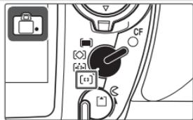
**2.3** Rotate the focus-mode selector until it clicks into place pointing to **S** (single-servo auto-focus). At this setting, the camera will focus automatically when the shutter-release button is pressed halfway. Pictures can only be taken when the camera is in focus.
