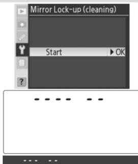
**3** Press the shutter-release button all the way down. The mirror will be raised and the shutter curtain will open, revealing the low-pass filter, and a row of dashes will blink in the control panel. The display in the viewfinder will turn off.
