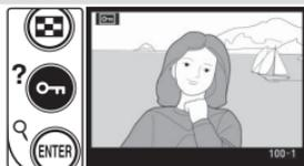
To remove protection from the photograph so that it can be deleted, display the photograph or highlight it in the thumbnail list and then press the
