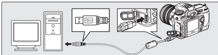
4 Turn the camera on. If **Mass Storage** is selected for **USB**, **PC** will be displayed in the control panel and viewfinder, and the PC mode indicator will flash (if **PTP** is selected, the camera displays will not change). Photographs can be transferred to the computer as described in the manual for the supplied software (on CD).
