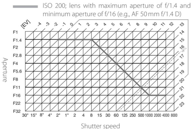
The maximum and minimum values for EV vary with sensitivity (ISO equivalency); the above graph assumes a sensitivity of ISO 200 equivalent. When matrix metering is used, values over 16 $\frac{2}{3}$  EV are reduced to 16 $\frac{2}{3}$  EV.
