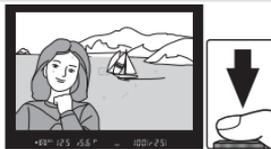
In single-servo AF, focus will remain locked between shots as long as the shutter-release button is kept pressed halfway, allowing several photographs in succession to be taken at the same focus setting. Focus will also remain locked between shots while the **AE-L/AF-L** button is pressed.
