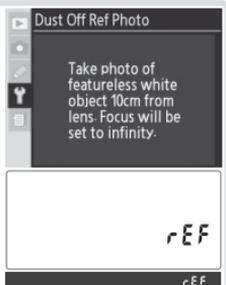
**3** With the lens ten centimeters (four inches) from a bright, featureless white object, frame the object so that nothing else is visible in the viewfinder and press the shutter-release button halfway. In autofocus mode, focus will automatically be set to infinity; in manual focus mode, set focus to infinity manually before pressing the shutter-release button. If using the aperture ring to set aperture, choose the minimum setting (largest f/-number).
