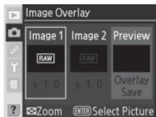
**3** Press the **ENTER** button to view the RAW images on the memory card. Press the multi selector left or right to highlight images. To zoom in on the highlighted image, press and hold the **📷** button.
