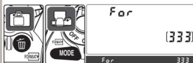
Turn camera on and press **FORMAT** (Ⓜ) and **MODE** buttons simultaneously for about 2 seconds until **F a r** blinks in control panel and viewfinder.
