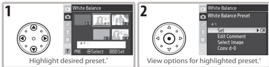
\* To set white balance to the value for the highlighted preset and return to shooting mode without completing Step 2, press **OK** button.
