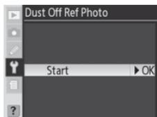
**1** Mount a CPU lens on the camera (a lens with a focal length of at least 50 mm is recommended). The **Dust Off Ref Photo** option is only available with CPU lenses. If using a zoom lens, zoom in to the maximum telephoto position.
