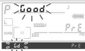
If lighting is too dark or too bright, the camera may be unable to measure white balance. A flashing **no Good** will appear in the control panel and viewfinder for about three seconds. Return to Step 4 and measure white balance again.
