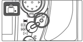
2 Turn the camera off and open the memory card slot cover.
