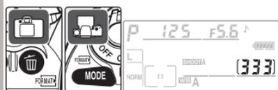
Press **FORMAT** buttons again.\* Do not turn camera off or remove battery or memory card until formatting is complete and control panel shows number of exposures remaining.
