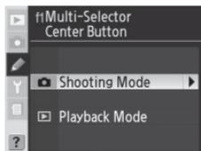
**Shooting Mode:** This option controls what operation can be performed by pressing the center of the multi selector when the camera is in shooting mode.
