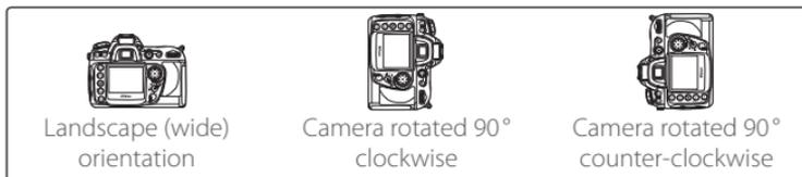
\* In continuous mode (P. 26), orientation recorded for first shot applies to all images in same burst, even if camera orientation is changed during shooting.
