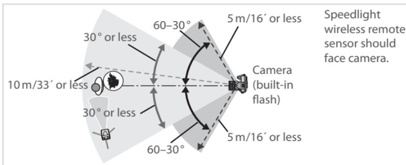
Maximum distance between optional Speedlights and camera is about 10 m (33') when Speedlight is positioned in front of camera (within 30° on either side of center line), or about 5 m (16') when Speedlight is 30–60° to either side of center line.
