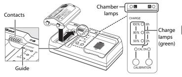
Insert the battery (terminals first), aligning the end of the battery with the guide and then sliding the battery in the direction indicated until it clicks into place. The chamber lamp and charge lamps will blink while the battery charges:
