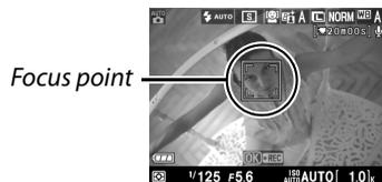
**Wide area and normal area:** Use the multi selector to move the focus point to any point in the frame.
