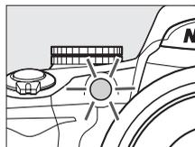
The timer will not start if the camera is unable to focus or in other situations in which the shutter can not be released.
