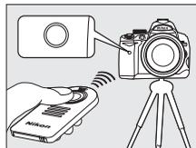
If no operations are performed for about a minute after selecting delayed remote or quick-response remote modes, the camera will automatically return to single frame, continuous, or quiet shutter-release mode, cancelling remote control mode.
