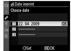
To choose a date counter format, highlight **Display options** and press **▶** to display the menu shown at right. Highlight an option and press **OK**. Highlight **Done** in the date counter menu and press **OK** when settings are complete.
