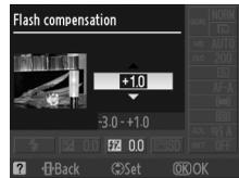
Normal flash output can be restored by setting flash compensation to  $\pm 0.0$ . Flash compensation is not reset when the camera is turned off.
