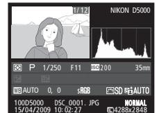
To end playback and return to shooting mode, press the shutter-release button halfway.
