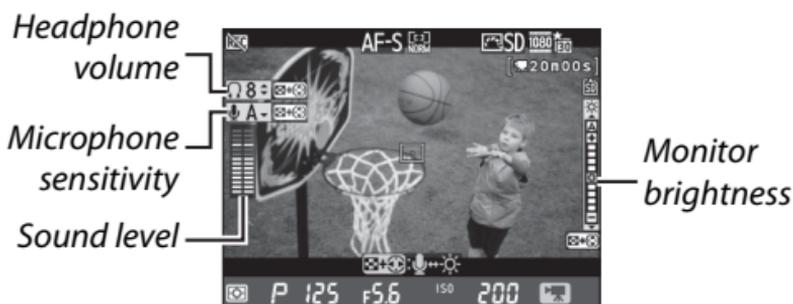
Note that microphone sensitivity and headphone volume can not be adjusted during recording, and that brightness applies to the display in the monitor only and has no effect on movies.
