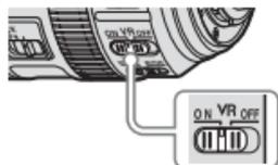
If the lens has a vibration reduction mode switch, choose **NORMAL** for hand-held photography or when using a monopod. Vibration reduction should generally be turned off when the camera is on a tripod, although an exception can be made for a lens such as the AF-S NIKKOR 200mm f/2G ED VR II, which automatically detects tripod vibration. Vibration reduction should also be turned off if you notice shake during filming when panning a camera that is mounted on a tripod.
