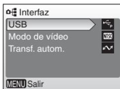
**5** Pulse **▲** o **▼** para seleccionar [PTP] o [Mass storage] y pulse **OK**.
