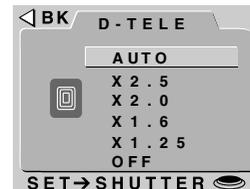
Digital-zoom settings only take effect when the LCD monitor is on. While digital zoom is in effect, the zoom indicator will be displayed in the LCD monitor, with the digital-zoom ratio shown to its right, and the green AF lamp will blink slowly. To restore automatic digital zoom, select AUTO from the D-TELE menu.
