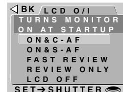
The chosen setting affects M-REC mode only. The LCD monitor will always come on when the mode dial is turned from OFF to A-REC or PLAY.
