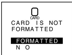
The card has not been formatted for use in the COOLPIX 950. Highlight FORMAT and press the shutter-release button to format the card, erasing any data that may be present, or turn the camera off and replace the card. If you select NO, you will not be able to record or playback photographs until the card has been formatted or replaced.
