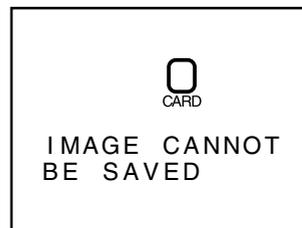
The camera has encountered an error while saving a photo or has run out of file numbers in the current folder. Try saving photos to a different folder. If the SEQ.XFER option is on, choose OFF or RESET from the SEQ.XFER menu (see "The Camera Menu: The M-REC Menu"). If the error persists, it may indicate that the card is not properly formatted. Transfer all photographs stored on the card to a computer and format the card as described in "The Camera Menu: The A-REC Menu."
