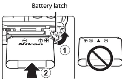
**✓** **Inserting the Battery Correctly**
