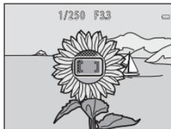
**3** Continue holding down the shutter-release button halfway and recompose the picture.
