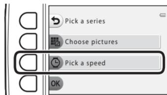
**4** Press flexible button 2 (**Fast**), flexible button 3 (**Normal**) (default setting), or flexible button 4 (**Slow**) to select a desired speed.
