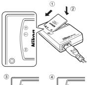
CHARGE lamp starts blinking when battery is inserted ③. Charging is complete when lamp stops blinking ④.
