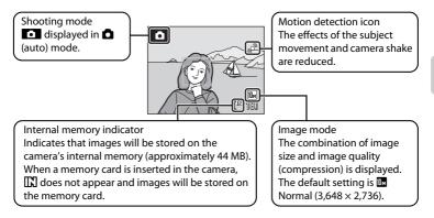
The indicators and photo info displayed during shooting and playback will turn off after a few seconds ( $\square$  118). When the monitor has turned off in standby mode to save power, press the power switch or the shutter-release button to reactivate it ( $\square$  122).
