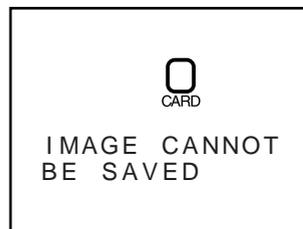
This error occurs when the card contains a photograph with the filename "9999.JPG." The file "9999.JPG" must be deleted before more photographs can be taken. If the error persists, transfer all photographs stored on the card to a computer and format the card as described in *"Advanced Settings: Formatting Memory Cards."*
