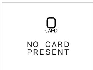
The camera can not detect a flash-memory card. Turn the selector dial to OFF and confirm that the flash-memory card has been correctly inserted in the camera as described in *"First Steps: Inserting and Removing Memory Cards."*
