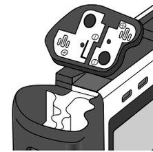
Use only 1.5V AA (LR-6) batteries (alkaline batteries are recommended, but nickel-cadmium, nickel metal-hydride, and lithium batteries may also be used) and be sure that all batteries are of the same type and model; do not mix batteries of different types or use new batteries together with old. Avoid using old batteries, as the battery indicator may not be able to display their level accurately. Once the batteries have been replaced, close the cover and slide it back until it latches.
