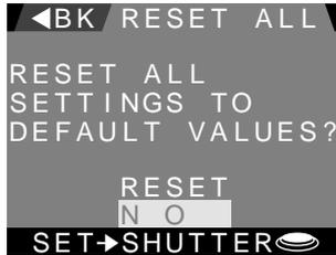
Highlight **RESET** and press the shutter button to restore settings to the following default values:
