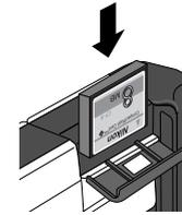
**Caution:** Be sure to insert the card as shown in the illustration, with the connectors towards the bottom of the slot and the label facing out. Inserting the card upside-down or backwards could result in damage to the camera or to the card.
