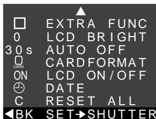
The shooting menu has two pages. Use the zoom-out (W/▼) and zoom-in (T/▲) switches to highlight the desired menu item. Pressing the zoom-out switch when the last item on a page is highlighted (or pressing the zoom-in switch when the first item is highlighted) displays the next page of items. To edit a highlighted item, press the shutter button. Press the MENU button to exit the shooting menu, or highlight ◀BK and press the shutter button.
