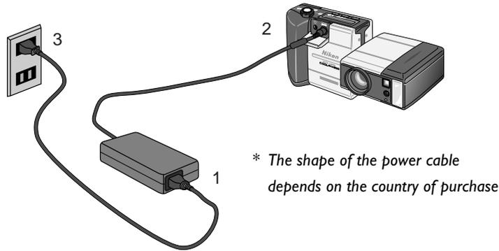
Plug the power cable into a power outlet. You are now ready to turn the camera on.
