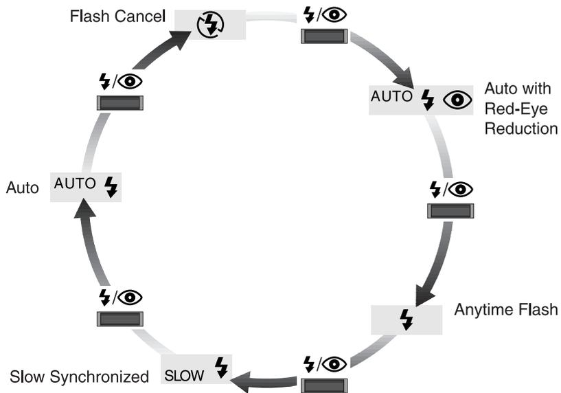
**Note:** The current flash mode is stored in memory when the camera is turned off and will be restored when the camera is next turned on.
