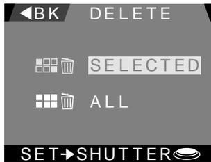
To select multiple photographs for deletion, highlight **SELECTED** and press the shutter button. The window shown below will appear.
