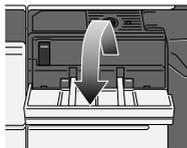
Insert the card as shown below, sliding it in until it is firmly in place at the back of the slot.
