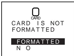
The card has not been formatted for use by the COOLPIX 900. Highlight **FORMATTED** and press the shutter button to format the current card (this will permanently erase any data on the card), or turn the camera off and replace the card. If **NO** is selected, although the camera will
