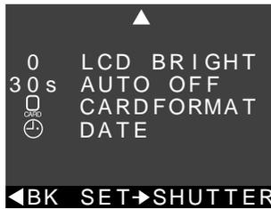
The playback menu has two pages. Use the zoom-out (W/▼) and zoom-in (T/▲) switches to highlight the desired menu item. Pressing the zoom-out switch when the last item on a page is highlighted (or pressing the zoom-in switch when the first item is highlighted) displays the next page of items. To edit a highlighted item, press the shutter button. To exit the playback menu, press the MENU button or highlight ◀BK and press the shutter button.
