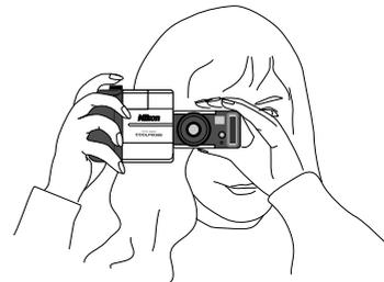
**Note:** Be sure that the lens and flash window are not obstructed by your fingers, hair, the camera strap, power cord, or video cable.
