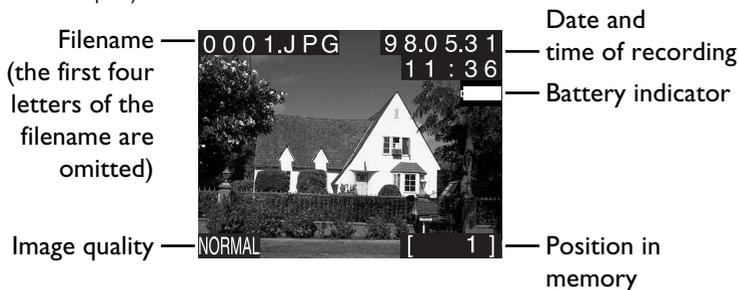
The filename, date-of-recording, and other indicators can be hidden by pressing the MONITOR button. To view the indicators once more, press the MONITOR button until they reappear. If no operations are performed for thirty seconds, the monitor will go off automatically to save power. To turn the monitor on again, press the MONITOR or shutter button. The length of time before the monitor goes off automatically during playback can be set using the playback menu. See “**Auto Off**,” below.
