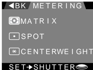
Highlight the desired metering method and press the shutter button. The current metering method is shown by an icon in the control panel and shooting menu and, when the camera is in M-REC mode and the metering method is **SPOT** or **CENTERWEIGHT**, in the color LCD monitor.
