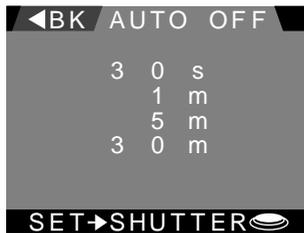
Settings of thirty seconds, one minute, five minutes, and thirty minutes are available. Highlight the desired setting and press the shutter button to put the change into effect, or highlight **<BK** and press the shutter button to discard any changes and return to the shooting menu. Pressing the MENU button will return you to M-REC mode.
