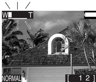
Because the viewfinder does not reflect the effects of digital zoom, it is recommended that you frame photographs in the monitor when digital zoom is in effect. Digital zoom is only in effect when the color LCD monitor is on. Turning the monitor off by pressing the MONITOR button returns the camera to ordinary optical zoom mode. Digital zoom will be restored when the monitor is turned on once more.
