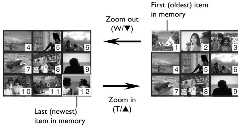
Once the desired photograph has been selected, press the shutter button to view it at full size.
