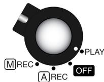
Turning the selector dial to PLAY causes an hourglass icon (⌚) to be displayed in the color LCD monitor while the camera reads the most recently recorded photograph from memory and displays it in the monitor (if there is no card in the camera or the card currently in the camera contains no images or is not formatted, an error message will be displayed; error messages are described in “**Troubleshooting**,” below). The camera’s playback display is shown below.
