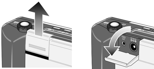
Connect the cable to the camera by inserting the black plug into the video jack. The cable can be connected when both the camera and television are on or when either or both are off.
