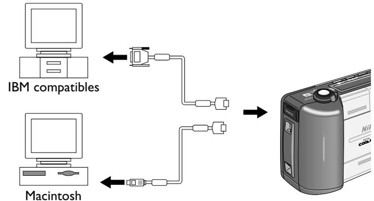
**Note:** When connecting the COOLPIX 900 to a computer, use only the cables provided with the camera. The COOLPIX 900 comes with a 9-pin RS-232C serial cable for connection to a male 9-pin serial connector, standard on many IBM-compatible computers, and a mini DIN 8-pin RS-232/RS-422 serial cable for connection to Macintosh computers. Use the cable appropriate to your computer.
