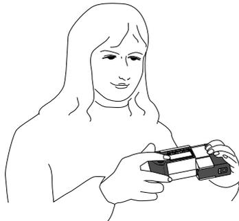
**Note:** In self-portrait mode (with the lens rotated to point at the user), a mirror image of the view through the lens will be shown in the monitor and camera settings will be hidden. Photographs taken in this mode will not however be reversed.
