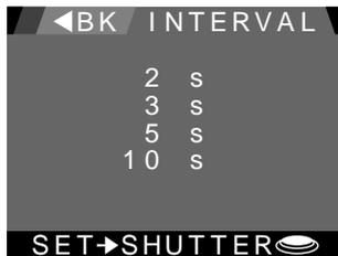
Change the interval setting by highlighting the desired interval and pressing the shutter button, or highlight **◀BK** and press the shutter button to leave the interval unchanged. Either action will return you to the slideshow menu shown above. While an interval setting is highlighted, it will blink at the same rate as the selected value.
