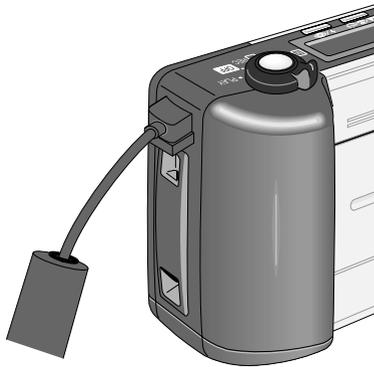
Attach the other end of the cable to the computer's serial port (IBM compatibles) or printer or modem port (Macintosh).
