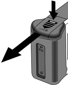
Insert the batteries with the positive (+) and negative (-) poles aligned as shown in the label at the entry to the battery chamber.
