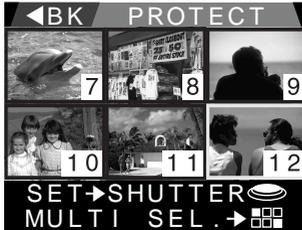
Using the zoom switch, highlight a photograph that you would like to protect. Images not currently visible will appear when the zoom switch is used to scroll past the first or last item in the window. Photographs that have been hidden with **HIDE IMAGE** will not be displayed and consequently cannot be protected using this option. Hidden images however cannot be selected and are thus protected from deletion.
