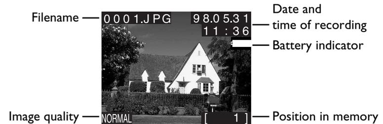
If nothing shows in the monitor, press the MONITOR button until the photograph and related information are displayed; pressing the MONITOR button once more will hide the image information and battery indicator, leaving only the photograph displayed.
