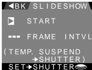
By default, each photograph in the slideshow will be displayed three seconds (depending on the length of time need to read the photograph from memory and first display it on the monitor, the length of time photographs are displayed may vary slightly). To set the length of time each photograph will be displayed, highlight **FRAME INTVL** (frame interval) and press the shutter button. The menu shown below will appear.
