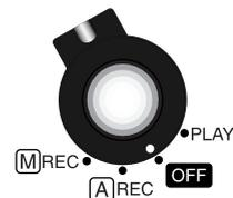
The camera is off when the control panel display is blank; if the monitor is off but the control panel is on, the camera has not been turned off. Check that the camera is off before putting it away.
