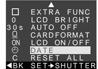
Press the zoom-out switch (W/▼) until the **DATE** item in the second page of the shooting menu is selected as shown above at right, then press the shutter button to display the date menu.
