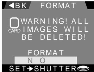
Press the zoom-in switch (T/▲) to highlight **FORMAT**, then press the shutter button. The following message will be displayed while the memory card is being formatted.
