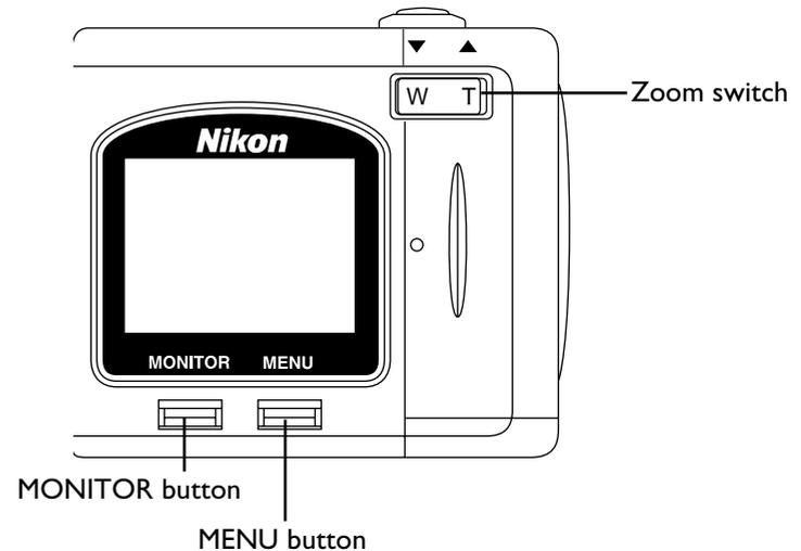
When the monitor is on and camera settings are displayed, pressing the MONITOR button will hide the camera settings. Pressing the button a second time will turn the monitor off. To turn the monitor on, press the MONITOR button once.
