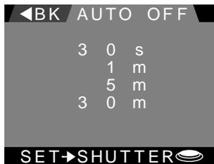
Settings of thirty seconds, one minute, five minutes, and thirty minutes are available. Highlight the desired setting and press the shutter button to put the change into effect, or highlight **<BK** and press the shutter button to discard any changes and return to the playback menu. Pressing the MENU button will return you to playback mode.
