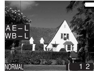
**Note:** *When autoexposure lock is in effect, the flash will automatically be set to “Flash Cancel” and will not fire even when lighting is inadequate.*
