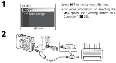
After confirming that the camera is off, connect the UC-E6 USB cable as shown above
