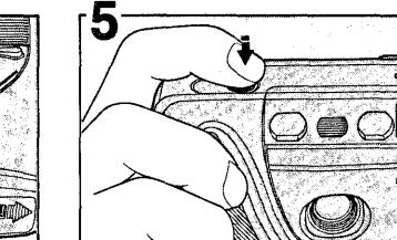
Lightly press shutter release button and confirm focus/focus memory indicator LED lights up to indicate sufficient battery power.
