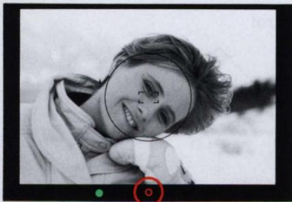
4. Rotate either shutter speed dial or aperture dial until exposure indicator LED lights up.
