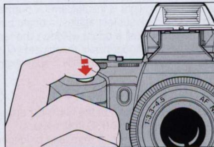
2. Lightly press shutter release button to turn on the N4004s.
