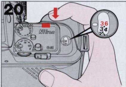
The film advance stops automatically at the end of the roll. Then, the self-timer indicator LED lights up for a few seconds and the shutter locks.
