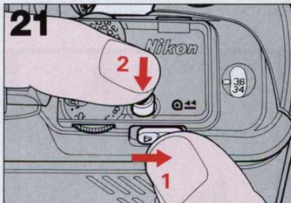
While sliding film rewind lever, push the film rewind button.
