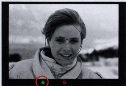
4. Keeping the shutter release button lightly pressed, watch the focus indicator LED in the viewfinder and rotate the lens focusing ring manually until the focus indicator LED lights up.
