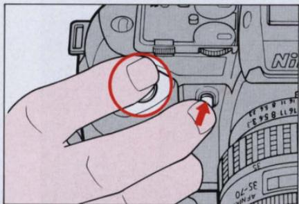
3. While lightly pressing shutter release button, depress the AEL button and hold it in.
