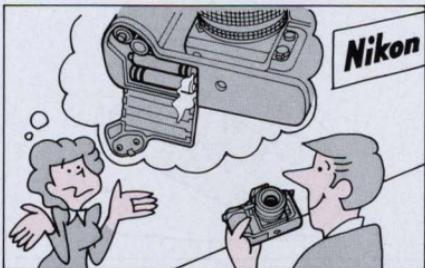
5. If the battery chamber is contaminated by battery leakage, take the camera to an authorized Nikon dealer.
