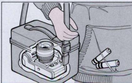
2. Battery power falls off in extremely cold temperatures—make sure batteries are new and keep the camera body wrapped in something warm.
