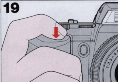
19 Fully depress shutter release button to take picture. This automatically advances film by one frame.
