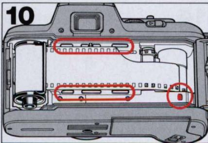
**10** Check to make sure film is positioned properly, with no slack.
