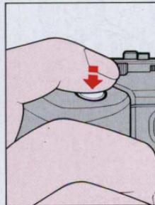
1. Center the focus brackets on the subject and lightly press the shutter release button.
