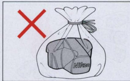
desiccant to keep out dust, moisture and salt. Note, however, that storing the leather case in a vinyl bag may cause the leather to deteriorate.
