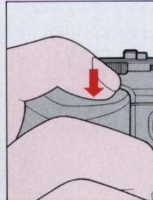
3. Keeping the shutter release button lightly pressed, recompose and fully depress the shutter release button.
