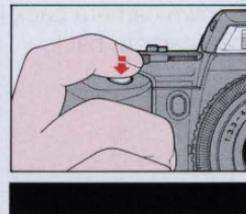
If LED goes off approx. 2 sec. after finger is removed from button, batteries need replacement.
