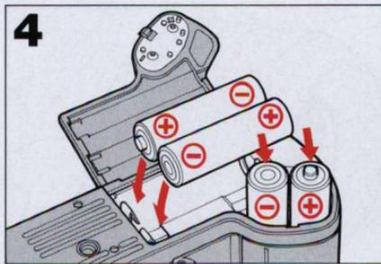
Install four fresh AA-type batteries with “+” and “-” ends positioned as shown inside the battery chamber.
