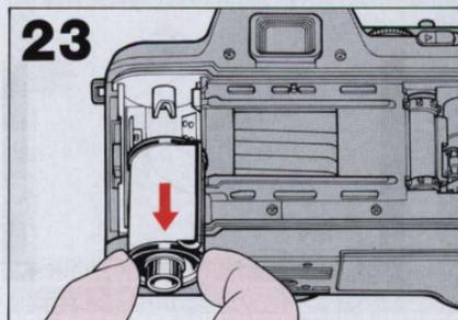
Open camera back and remove film cartridge.
