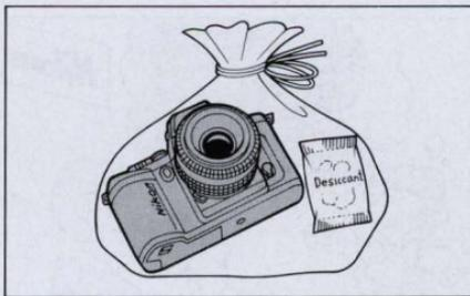
**10.** Store the camera in a cool, dry place away from naphthalene or camphor (moth repellents). In a humid environment, store the camera inside a vinyl bag with a
