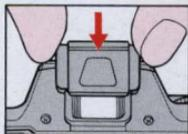
In program, shutter-priority, or aperture-priority auto exposure mode, use eyepiece cover DK-5 to prevent stray light from entering the viewfinder.
