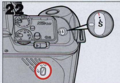
After rewinding stops (automatic), confirm film frame counter has returned to "S".
