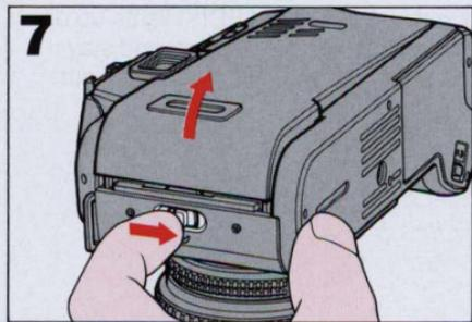
Slide down camera back lock release to open camera back.
