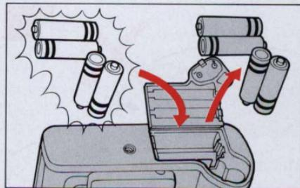
3. When replacing batteries, be sure to replace all batteries at the same time. Always use fresh batteries of the same brand.
