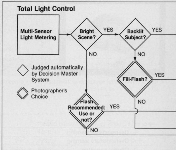
In short, just by composing the picture and pressing the shutter release, the N4004s automatically gives you excellent results, even in difficult lighting situations which might otherwise require complicated exposure techniques.
