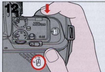
**12** Fully depress shutter release button to automatically advance film to frame "1." Observe film advance indicator rotation to confirm proper film installation and transport.
