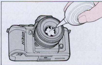
8. Clean glass surfaces such as the lens with a blower brush; avoid using lens tissue as much as possible. To remove dirt and smudges, use soft cotton moistened with pure alcohol and wipe
