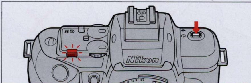
2. Press self-timer button. Self-timer indicator LED starts blinking and shutter is released after approx. 10 sec. For final two seconds, the LED lights up.
