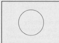
In manual exposure mode or when the AEL button is used in program, shutter-priority or aperture-priority auto exposure mode, the camera automatically switches to centerweighted metering. Centerweighted metering places special emphasis on brightness within the 12mm-diameter central area of the viewfinder, and is recommended for creating special effects.
