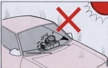
**4.** Do not leave the camera in an excessively hot place.
