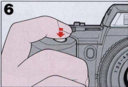
Lightly press shutter release button and check viewfinder exposure indicator LED(s) to make sure battery power is sufficient.
