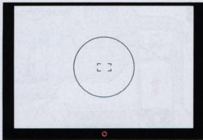
Exposure indicator LED(s) lights up or blinks if power is sufficient, and stays on approx. 8 sec. after you take your finger off the button.
