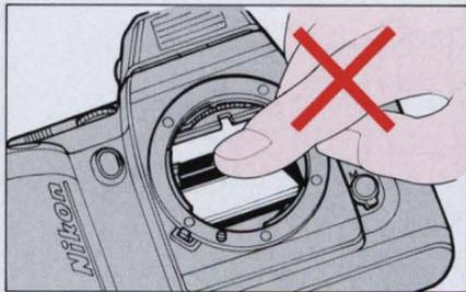
1. Never touch the reflex mirror, focusing screen or AF contacts. Remove dust with a blower brush.
