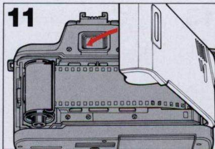
**11** Close camera back and confirm lock-release snaps closed.
