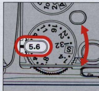
2. Adjust the shutter speed and aperture for correct exposure.
