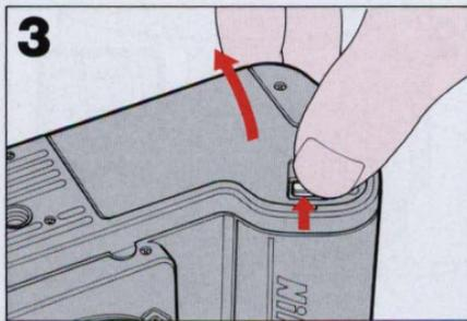
Open the battery chamber lid by sliding the lock release.
