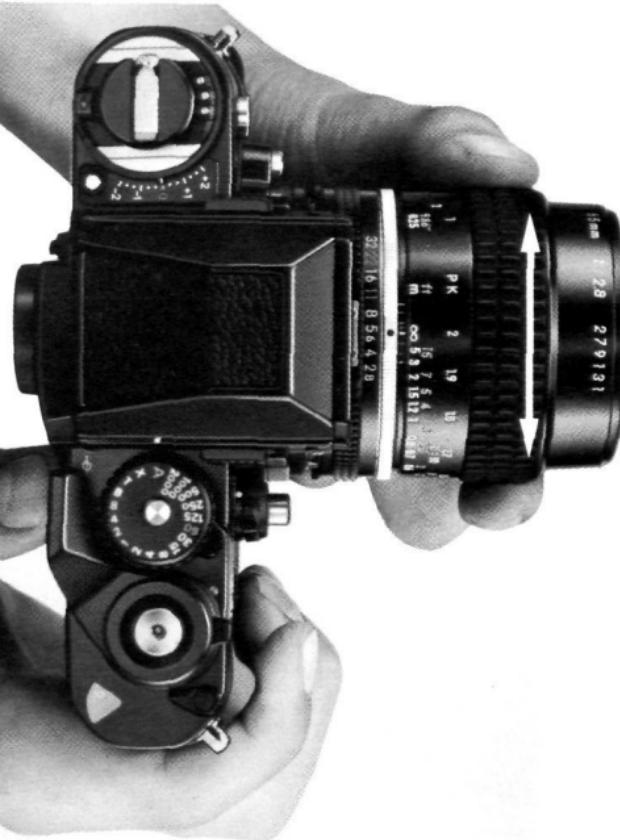
Thanks to its fully automatic diaphragm, the Micro-Nikkor can be focused with maximum image brightness on the screen throughout the entire focusing range. The depth of field is also minimized at maximum aperture, so that the image snaps in and out of focus rapidly and distinctly.
