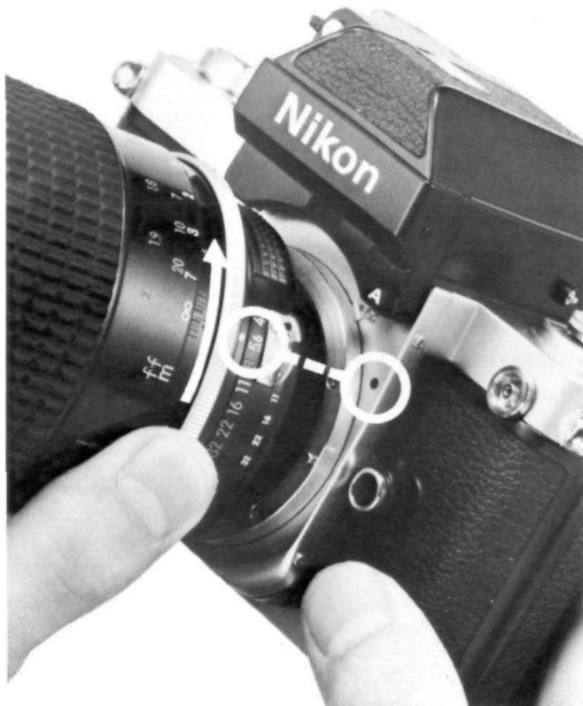
Position the lens in the camera's bayonet mount, aligning the mounting indexes on the camera and the lens. Twist the lens counter-clockwise until it clicks into place.
