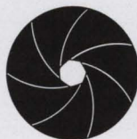
Lens at f/16 : Sharp focus is extended to encompass the entire foreground and background.
