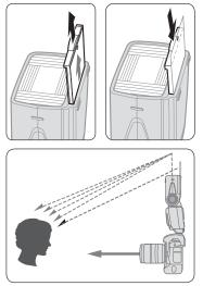
Pull out the bounce card and the built-in wide panel and, while holding the bounce card, slide the built-in wide panel back into place inside the flash head.
