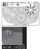
Make sure that the flashready indicator on the SB-910 or in the camera's viewfinder is on before taking a picture.
