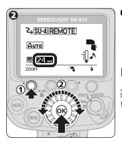
Press function button 1 to highlight the zoom head position, choose a zoom head position with the selector dial, and then press the [OK] button.
