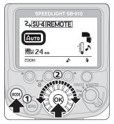
To set the flash mode, press the [MODE] button, choose the flash mode with the selector dial, and then press the [OK] button.
