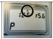
The D symbol above the shutter speed display indicates an active GPS Data Feed
