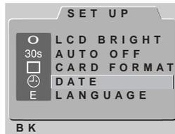
4 In the SET UP menu, use the zoom buttons (▲▼) to highlight DATE and press the shutter-release button to display the DATE menu.
