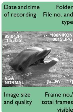
**4** If desired, you can zoom in on the current photo by pressing the  $\text{Q}/\text{⏏}$  button. The center portion of the image will be enlarged to fill the LCD monitor. Press the  $\text{Q}/\text{⏏}$  button once for a magnification of  $\times 2$ , twice for a magnification of  $\times 3$ . Press the  $\text{Q}/\text{⏏}$  button a third time to view the photograph at full size.
