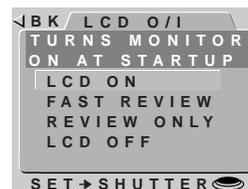
The chosen setting affects M-REC mode only. The LCD monitor will always come on when the mode dial is turned from OFF to A-REC or PLAY.
