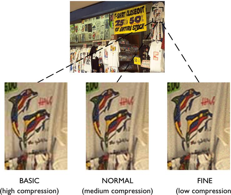
While a setting of NORMAL represents the best trade-off between memory and image quality in most cases, a setting of BASIC can be used to save memory. A setting of FINE is suitable for photographs that will be enlarged or printed at high resolution.
