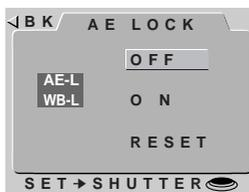
Autoexposure and white-balance settings are fixed at the values used in the first photograph taken after ON is selected. You can turn the lock function off to allow the camera to set autoexposure and white balance separately for each picture by selecting OFF from the AE-LOCK menu. To restore the original lock settings, select ON again. Before beginning a new panorama, select RESET to clear the previous settings, then repeat steps 2–5, above.
