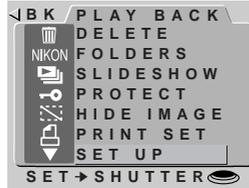
3 Using the zoom buttons (▲▼), highlight SET UP and press the shutter-release button.
