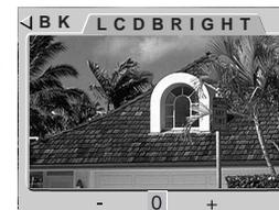
A setting of **-** will darken the display slightly, while **+** results in a slightly brighter display. These settings can not be used in combination; selecting **-** twice in a row will only darken the display by the same amount as selecting **-** once. Select **0** to restore normal brightness.
