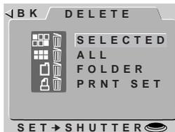
**2** Use the zoom buttons (▲▼) to highlight ALL and then press the shutter-release button. The dialog shown at right will be displayed. Highlight YES and press the shutter-release button to delete all visible, unprotected images. Highlight NO or BK to return to the playback menu without deleting the images.
