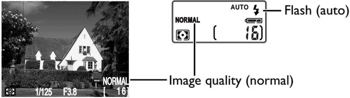
These settings allow the camera to set focus automatically at any distance greater than 30cm (one foot). The camera measures the available light and adjusts shutter speed and aperture accordingly, firing the flash to provide additional light as necessary.
