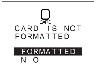
The card has not been formatted for use in the COOLPIX 700. Highlight FORMAT and press the shutter-release button to format the card, erasing any data that may be present, or turn the camera off and replace the card. If you select NO, you will not be able to record or playback photographs until the card has been formatted or replaced.
