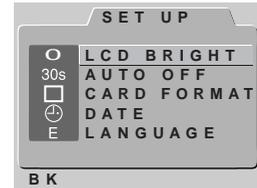
**AUTO OFF:** When operated on battery power, the camera automatically enters sleep mode if no operations are performed for thirty seconds. This option can be used to extend this limit for playback as described in “The Camera Menus: The A-REC menu,” above.
