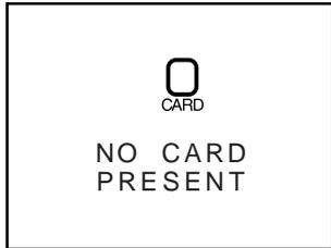
The camera can not detect a flash-memory card. Turn the mode dial to OFF and confirm that the flash-memory card has been correctly inserted in the camera as described in "First Steps: Inserting and Removing Memory Cards."
