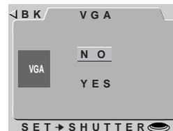
If an image size of 640 × 480 pixels is selected, a VGA indicator will appear in the LCD monitor whenever the mode dial is set to M-REC.
