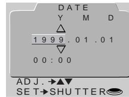
If the date has not been set, a flashing clock icon will appear at upper right in the LCD monitor when the mode dial is set to A-REC or M-REC. Photographs taken when this icon appears will have a time stamp of "99/01/01 00:00"; set the time and date as described above before shooting.
