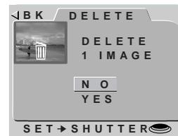
This dialog appears when the  $\text{⏏}$  button is pressed. Highlight YES using the zoom buttons (▲▼), then press the shutter-release button to delete the selected photograph. Select NO to return to playback mode leaving the photograph untouched.
