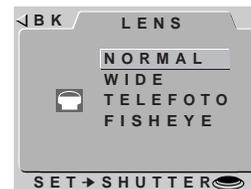
At settings other than NORMAL, a lens converter icon (📷) will appear in the LCD monitor, and settings will be optimized for the chosen converter as described at left. Choose NORMAL to cancel changes to settings and restore normal camera operation.
