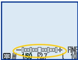
Control panel display is in EVs, rounded to nearest EV (display lasts for eight seconds after command dial is released, then is re-
