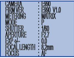
Camera type, firmware version, metering method, exposure mode, aperture, focal length, focus mode/distance
