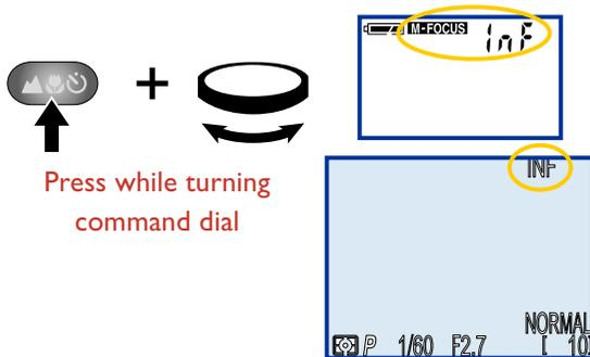
Focus distance is displayed in LCD monitor, and in control panel while command dial is rotated. After command dial is released, M-FOCUS icon in control panel indicates that manual
