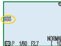
When photographs are taken with BSS on, the focus, exposure, and auto white-balance settings used for the first photo when the shutter-release button is pressed apply to all images in the series.
