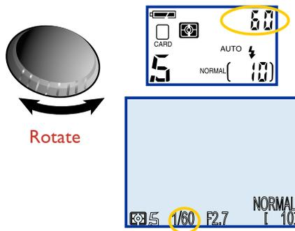
Shutter speed displayed in LCD monitor and control panel (shutter speeds of  $\frac{1}{4}$  s or more are shown in the LCD monitor in yellow to indicate that noise may appear in the final photograph)
