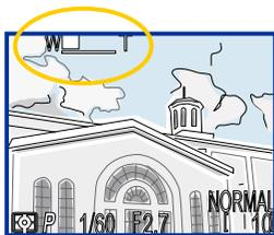
Indicator in LCD monitor displays amount of zoom while either button is pressed
