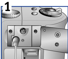
Connect UC-E1 USB cable to camera USB/serial connector
