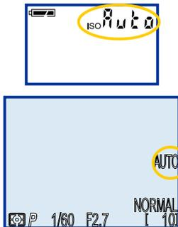
Sensitivity setting is displayed in LCD monitor, and in control panel while command dial is rotated. After command dial is released, ISO icon in control panel indicates that sensitivity adjustment is in effect.
