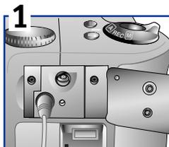
Connect SC-EM3 serial cable to camera USB/serial connector
