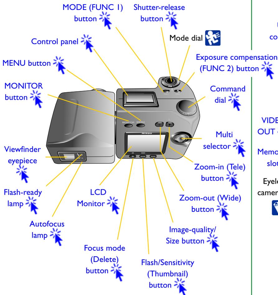
The lens section is attached to the camera body by a hinge that permits the lens to be rotated through 270°. For more information, see:
