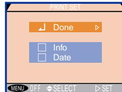
Menu of print set options displayed. To turn option on or off, highlight and press multi selector to right. Check **Date** to print date of recording on photo, **Info** to print shutter speed and aperture. Highlight **Done** and press multi selector to right to playback.
