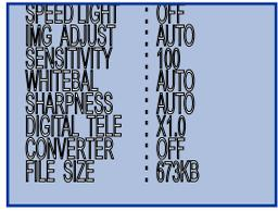
Flash on/off, image adjustment, sensitivity, white balance, sharpening, digital zoom, lens converter on/off, file size (kilobytes)
