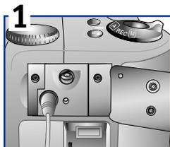
Connect SC-EW3 serial cable to camera USB/serial connector
