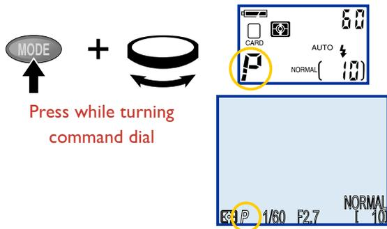
Confirm mode setting in control panel or LCD monitor
