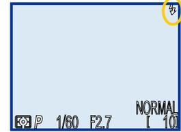
Confirm flash setting in control panel or LCD monitor (setting not displayed in monitor when flash set to “auto”)
