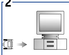
Connect cable to computer serial port
