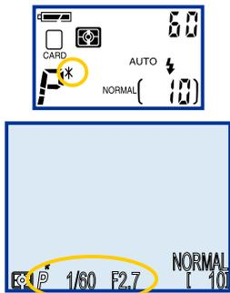
**P\*** appears in control panel and LCD monitor to indicate that flexible program is in effect. When monitor is on, values for shutter speed and aperture are displayed in control panel and LCD monitor (values are not displayed in control panel when monitor is off).
