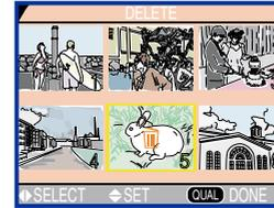
Press multi selector up or down to select image for deletion (selected images marked by icon). Repeat steps 1 and 2 to select more images. To deselect thumbnail, highlight and press multi selector up or down.
