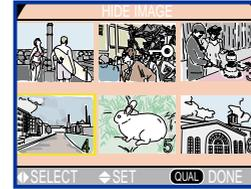
Press multi selector left or right to highlight desired thumbnail. To view more thumbnails, rotate command dial.
