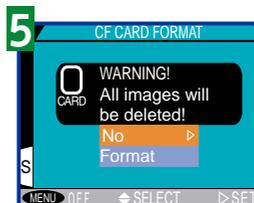
Confirmation dialog displayed. Press multi selector down to highlight **Format**, then press to right to format card. Do not turn camera off or remove card until "FORMATTING" message has disappeared from display. All data on card will be permanently deleted.
