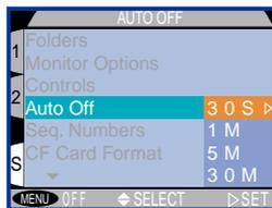
The time limit for playback is independent of the time limit for A-REC and M-REC, and is set by choosing **Auto Off** from the playback setup menu. The time limit for A-REC and M-REC can be set by choosing **Auto Off** from either of the A-REC or M-REC setup menus.
