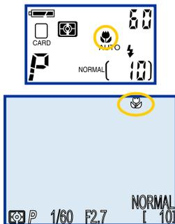
Confirm focus-mode setting in control panel or LCD monitor
