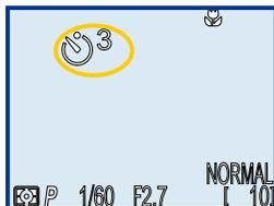
Count-down timer in LCD monitor shows number of seconds remaining to shutter release after shutter-release button fully pressed
