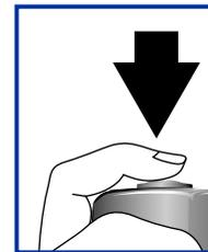
Do not change the distance between the camera and the subject while focus lock is in effect. If your subject moves, remove your finger from the shutter-release button and focus again at the new distance.
