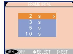
Owing to differences in the speed at which images can be read from the memory card, depending on the file size of the images in the slide show, the actual interval may differ from the value chosen in the interval menu.
