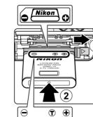
**Inserting the Battery**
