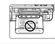
C Close the battery-chamber/memory card slot cover.
