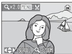
The magnification ratio can be changed further by operating the zoom buttons. The zoom ratio will be displayed in the monitor, and can be increased up to 10x. The following operations can be performed while pictures are zoomed in.
