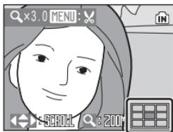
When using playback zoom with pictures shot using the face-priority function (94), the picture will be enlarged, with the face recognized during shooting, at the center of the monitor. If more than one face was recognized, the picture would be enlarged with the face, on which focus was acquired, at the center of the monitor. Press the multi selector ▲, ▼, ◀, or ▶ to display a different recognized face.
