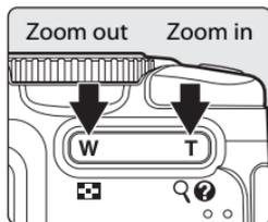
When the camera is zoomed in to the maximum magnification (3.6x), holding down **T** (Q) triggers digital zoom. The subject is magnified up to 4x, for a total magnification of 14.4x.
