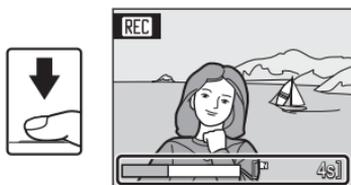
To end recording, press the shutter-release button all the way down a second time.
