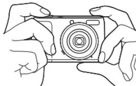
When taking pictures in “tall” orientation, turn the camera so that the built-in flash is above the lens.
