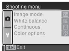
Press the multi selector **▲▼** to select a tab and press **OK** or **▶**.
