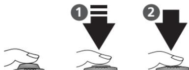
The COOLPIX5000 has a two-stage *shutter-release button*.
