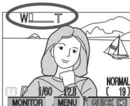
Indicator in monitor displays amount of zoom while either button is pressed
