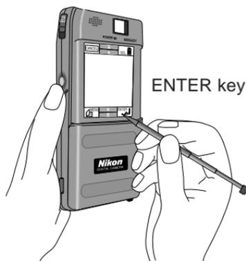
A beep will sound three times, signaling that the camera's electronic shutter has been released, and the READY lamp will blink while the camera transfers the photograph to memory. When the camera has finished recording the image, the exposure count in the status bar of the touch-panel display will go down by one.
