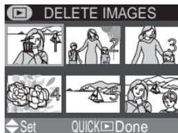
Press multi selector up or down to select picture for deletion. Selected pictures are marked by
