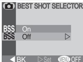
BSS may not produce the desired results with a moving subject or if you change the composition while the shutter-release button is pressed all the way down.
