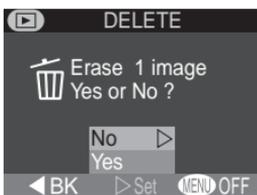
Press **QUICK** to display a confirmation dialog. Press multi selector up or down to highlight option, press to right to select:
