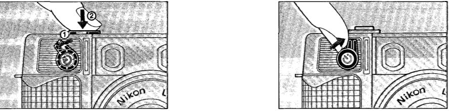
Turn the self-timer lever as far as it goes and depress the shutter release button. The shutter is released after approximately 10 seconds. Three seconds before the shutter is released, the indicator lamp starts blinking.
