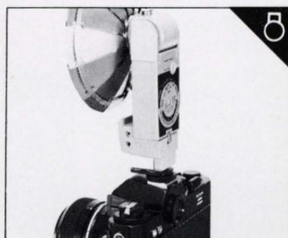
Remember that the camera's auto exposure control works only with constant light sources such as sunlight or photo floods and not with an instantaneous source such as a flashbulb or an electronic flash.
