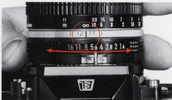
Guide to aperture setting using automatic exposure control
