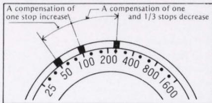
exposure, reset the green needle to a number higher or lower than the number indicated by the black needle in the shutter-speed scale.
