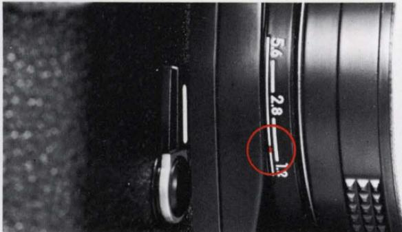
To remove the lens from the camera, press the lens-release button and twist the lens to the right as far as it will go. The lens will come loose and can be lifted out.
