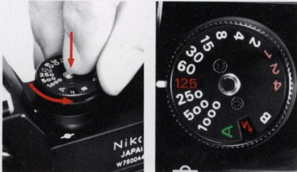
To make manual control, press the shutter speed dial lock in the center of the shutter speed dial, and turn the dial and align the desired shutter speed graduation to the indicator mark. In manual exposure control, intermediate speeds between graduations cannot be used.
