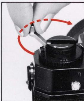
Unfold the rewind crank and turn it with a constant, gentle pressure in the direction of the arrow until you feel an increased tension. Give it a few more turns until the tension has gone and the crank turns freely. The film has now left the take-up spool and the camera may be opened.
